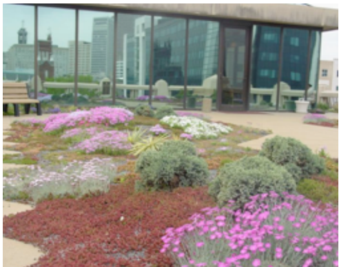
Example of an intensive green roof. Intensive green roofs require more maintenance and often feature plants and shrubs requiring more attention than extensive green roofs.
